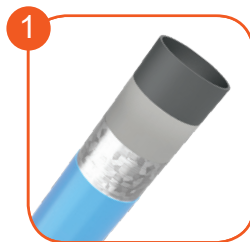
1 Solid construction made of black steel S235JR, cleaned in the sandblasting process. Protected against corrosion by galvanizing and powder coating with polyester paint QUALICOAT attested.
